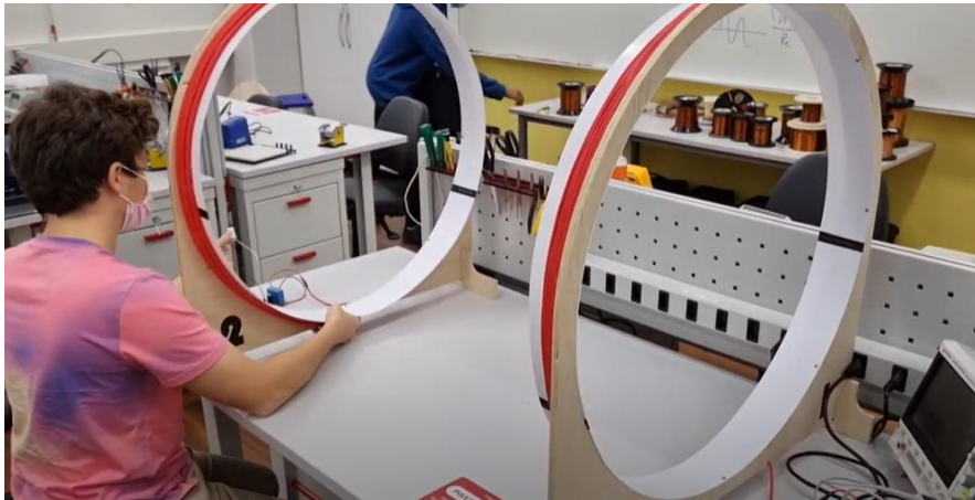
Figure 3. Physical setup for the WPT circuit shown in Figure 1 made by one of the groups.
