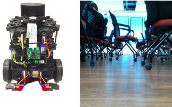
Figure 3. TB3 with the Raspcam installed and the display of the image captured by the robot camera.
