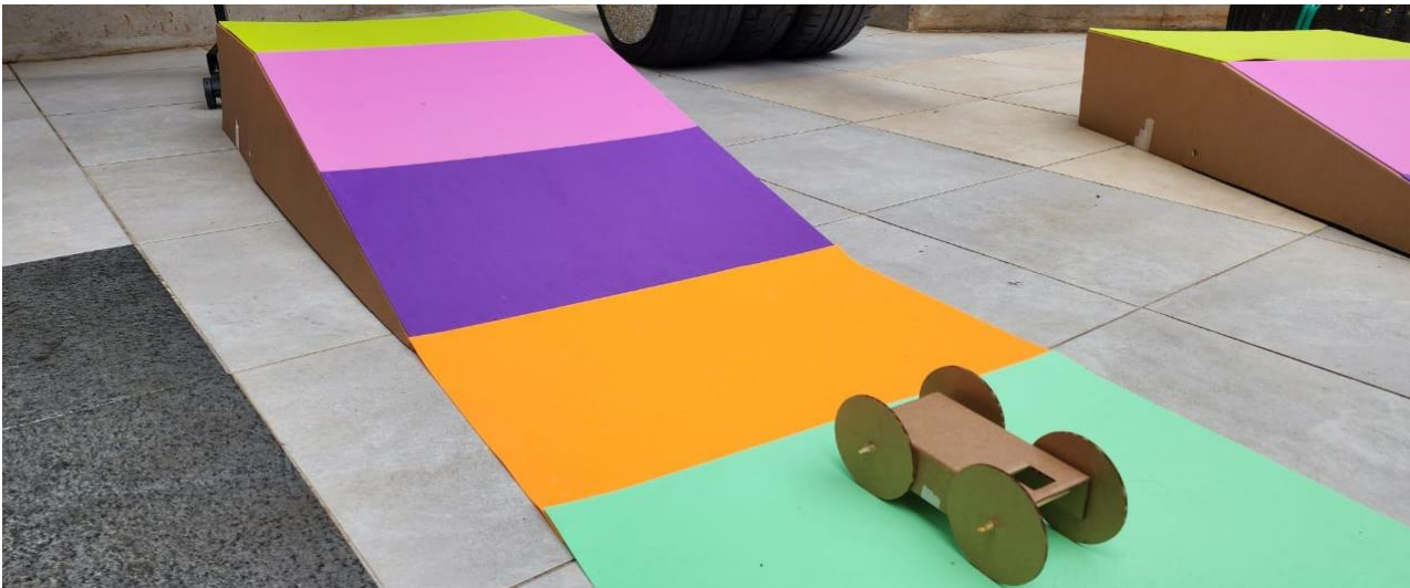
Figure 3. Car and ramp prototypes. The EVA foam cover on the ramp is recommended to increase friction.
