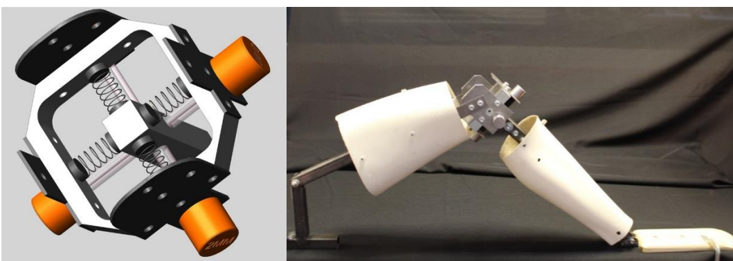
Figure 2. The mechanical design of the knee model (left) and the first prototype of the learning model (right).
